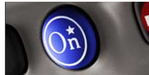
Figure 3: Within seconds of a moderate to severe crash, the OnStar module will send a message to the OnStar Call Center (OCC) through a cellular connection, informing the advisor that a crash has occurred. A voice connection between the advisor and the vehicle occupants is established. The advisor then can conference in 911 dispatch or a public safety answering point (PSAP), which determines if emergency services are necessary. If there is no response from the occupants, the advisor can provide the emergency dispatcher with the crash information from the SDM that reveals the severity of the crash. The dispatcher can identify what emergency services may be appropriate. Using the Global Positioning System (GPS) satellite, OnStar advisors are able to tell emergency workers the location of the vehicle.
