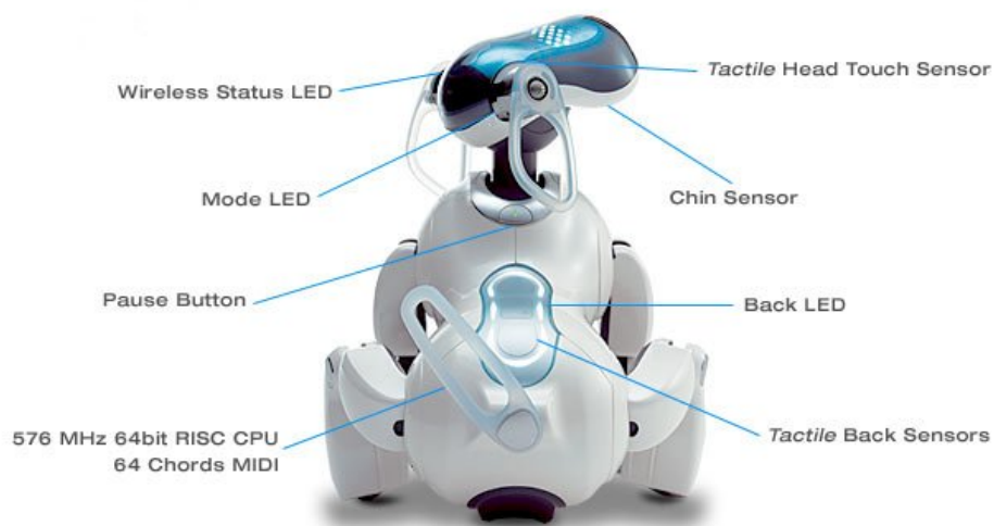
Figure 7 The hardware of the Aibo ERS7, rear view [source: Sony website]
